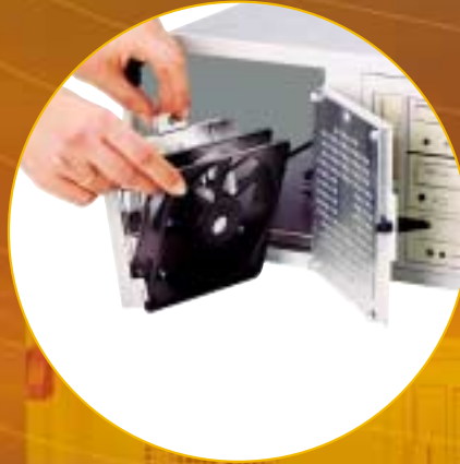
Fan can be pulled out from the front
