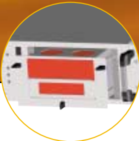
drive cage, can be pulled out quickly
