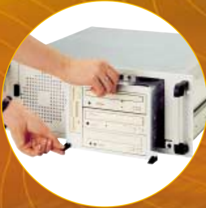
Drive cage can be pulled out from the front
